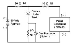
Notes: 1. Rise Time = 7 ns max. Input Impedance =1 M  $\Omega$  , 22 pF 2. Rise Time = 10 ns max. Input Impedance =  $50 \Omega$
