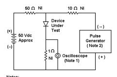
1. Rise Time = 7 ns max. Input Impedance =1 M  $\Omega$  , 22 pF
