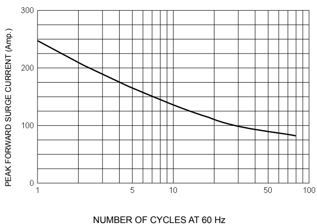
FIG-5 PEAK FORWARD SURGE CURRENT
