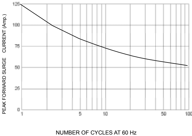
FIG-5 PEAK FORWARD SURGE CURRENT
