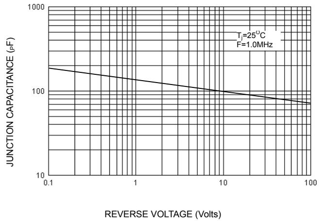
FIG-5 TYPICAL REVERSE CHARACTERISTICS Per leg
