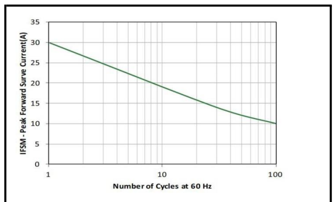
Figure 6 - Maximum Non-Repetitive Forward Surge Current Uni-Directional Only
